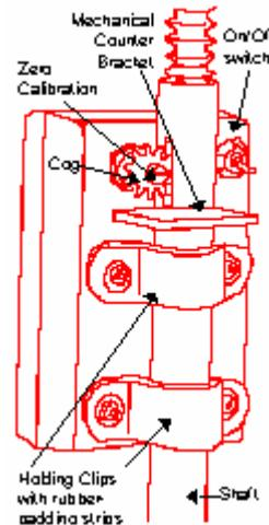
3. Lie the Electronic Plate Counter face down with the cog and the switch on the left. A table or workbench is ideal. Turn the cog on the Counter anti-clockwise (to the left) until it stops.
